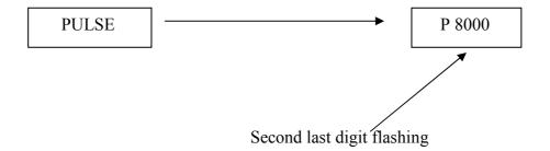
Start entering the pulse ratio immediately. The flashing digit can be changed by pushing the button in. Shortly after that digit is set, the next digit will flash and will be able to be set. This will continue until all digits have been set, at which point the display will change to the odometer or the trip meter reading.
